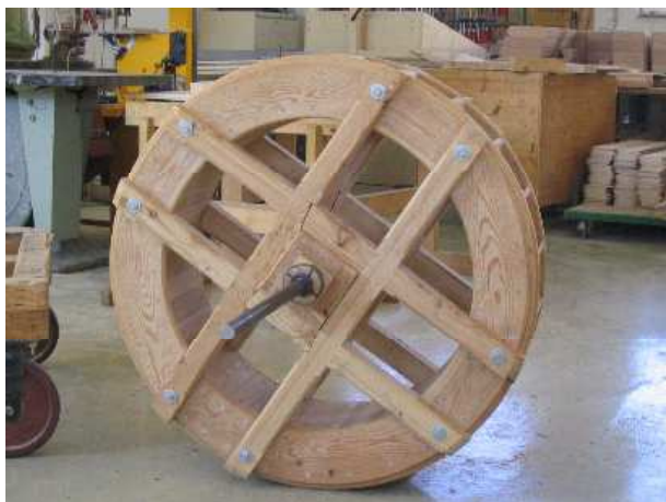
A traditional larch waterwheel made by GBL in Liezen
